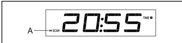
**To manually advance the scan cycle**, press the Multi-scan button repeatedly.
